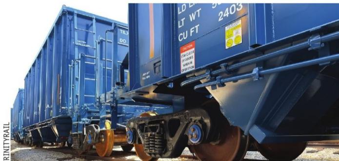
*TrinityRail*'s 2,403-cubic-foot rapid discharge triple hopper is equipped with three pneumatically operated discharge gates, featuring a transverse design to support versatile and efficient unloading operations for aggregates.
