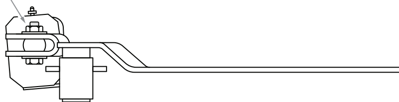
LOWER LOCK ARM INSTALLED (TOP VIEW)
